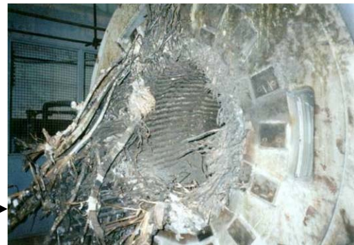
Figure 12 – Generator Catastrophic Failure
