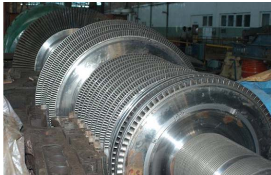
Figure 13 – Steam Turbine Rotor Reconditioned
