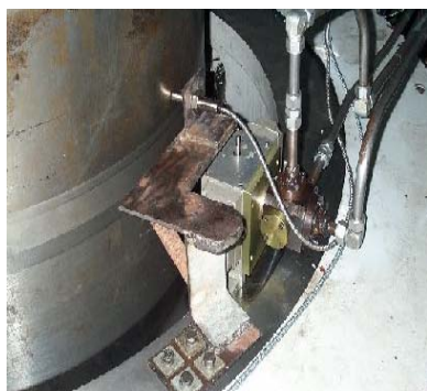
Eddy Current Probe for Shaft Position
