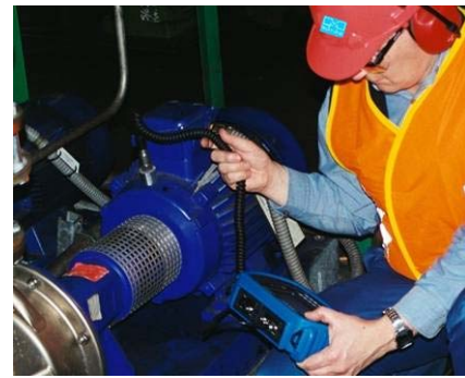
Figure 9 – Periodic Vibration Data Collection
