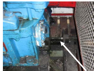
Figure 15.3 Findings: 18mm misalignment (1.6°) 5mm misalignment of chain sprockets Uneven chain running causing tooth wear.
