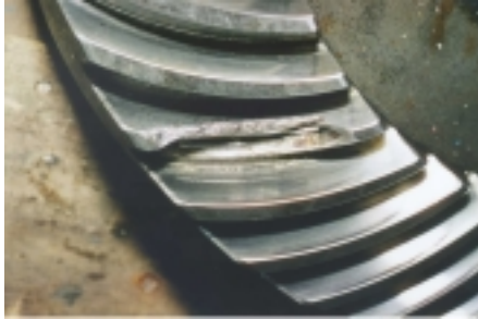
Figure 4: Damaged tooth on intermediate shaft bevel gear
